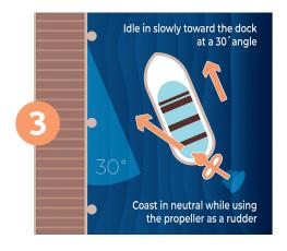
Docking is NOT a "cut and coast" maneuver. Reverse engine thrust is used to stop headway and assist with final positioning, as detailed in this graphic.
